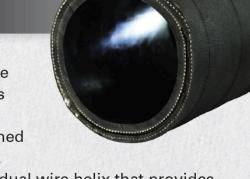
ethanol and gasoline. The hose construction incorporates a dual wire helix that provides full suction capability, kink resistance and a path to conduct a static electrical charge to ground. The cover is resistant to abrasion, heat, oil and weathering.
